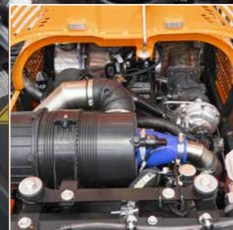
SILNIK YANMAR 60 KM STAGE V YANMAR ENGINE 60 HP STAGE V
